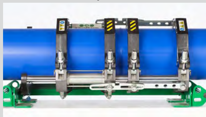
Join the pipes, cool under pressure.
