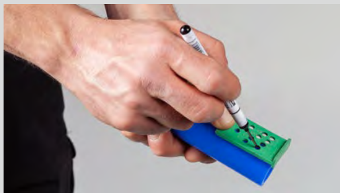
Marking of the welding depth
